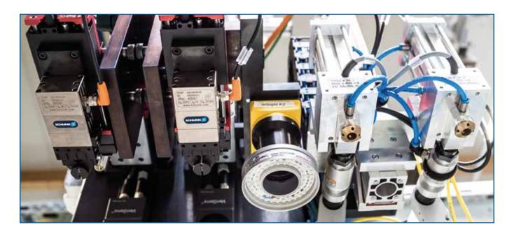
Feeding technology describes the process of feeding bulk materials into a setting operation in the correct position. This technology has been standard in HONSEL automation for years. Depending on the application and customer requirements, a fastener can be fed directly into the transfer unit of the setting device via a hose or without compressed air via a pick & place system.
