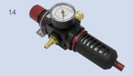
For BZ tools water trap / pressure reducer G3/8 filter regulator with filter pressure regulator, manometer, plastic protective cage, mounting bracket, G3/8 plug connection and quick-coupler.
